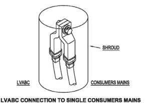
BOND CONNECTION 200/400 AMP (IF REQUIRED TO BE EQUIVALENT SIZE OF SERVICE MAINS) **FASCIA** SEE BELOW FOR SERVICE CONNECTION DETAIL EYEBOLT M16 (SWL 3.5kN) NON-METALLIC WEATHERPROOF LVABC **ENCLOSURE** MINIMUM SIZE 쭚 AS PER TABLE 5.1 LVABC CONSUMER MAINS BOND CONNECTION SEE NOTES
