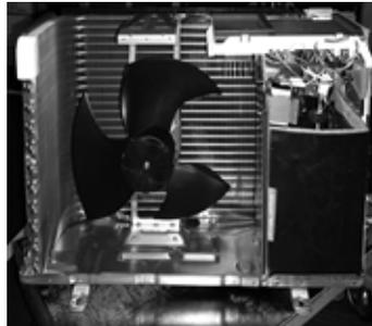
3. Remove all the connectors from Electrical Assembly.
