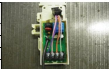
5. Fix Holder on terminal block support with the supplied screw.
