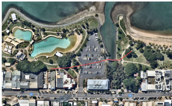
Fig 6 – Excavation route for the foreshore central carpark area.
