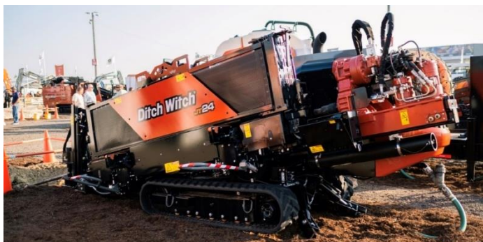
Fig 4 – Directional drilling rig will be used to bore under central carpark to install the electrical conduit.
