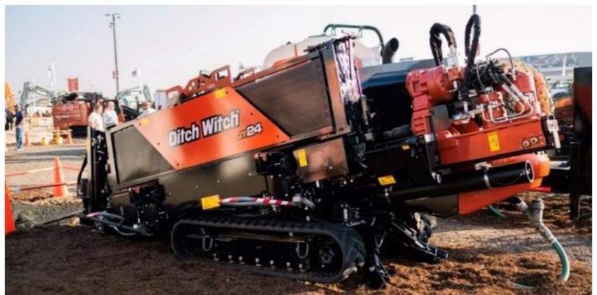
Figure 3 – An example of a directional driller completing underground excavation.
