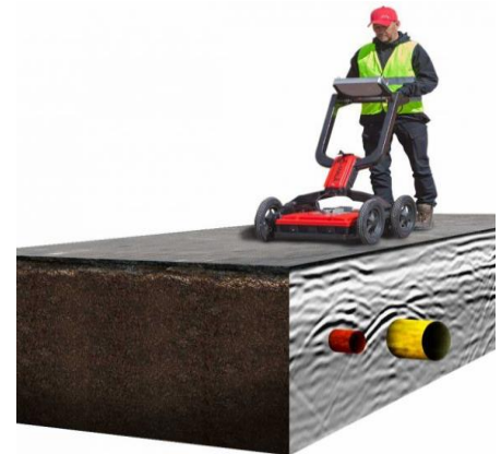
Figure 2 – An example of a ground penetrating radar identifying underground
