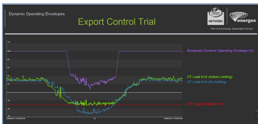
Figure 2: Demonstration of Dynamic Operating Envelope (purple line) used to manage reverse power flow through the local distribution transformer (green line)
