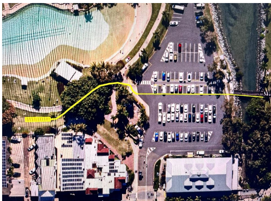
Fig 1 – Excavation route for the Foreshore Central Car Park area.
