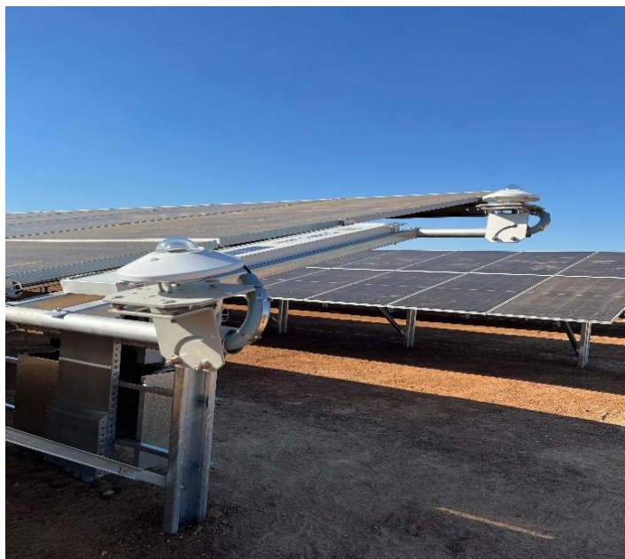
Weather sensors to monitor solar panel performance
