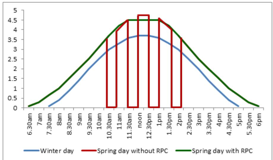
Fig 1 - Typical PV generation profiles (5kVA inverter)
