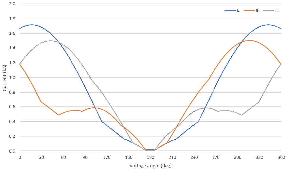
**Figure 12 – Transformer phase currents as a function of switching angle when energised against an ideal 66kV source with the worst residual flux**
