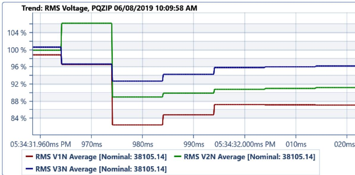
**Figure 18 - Measured 66kV rms voltages**
