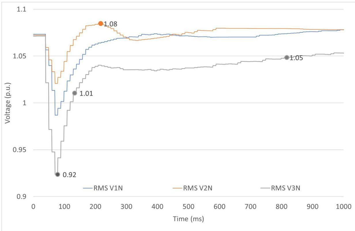
Figure 2- Demonstration of RMS Line-Neutral Voltages with worse case highlighted
