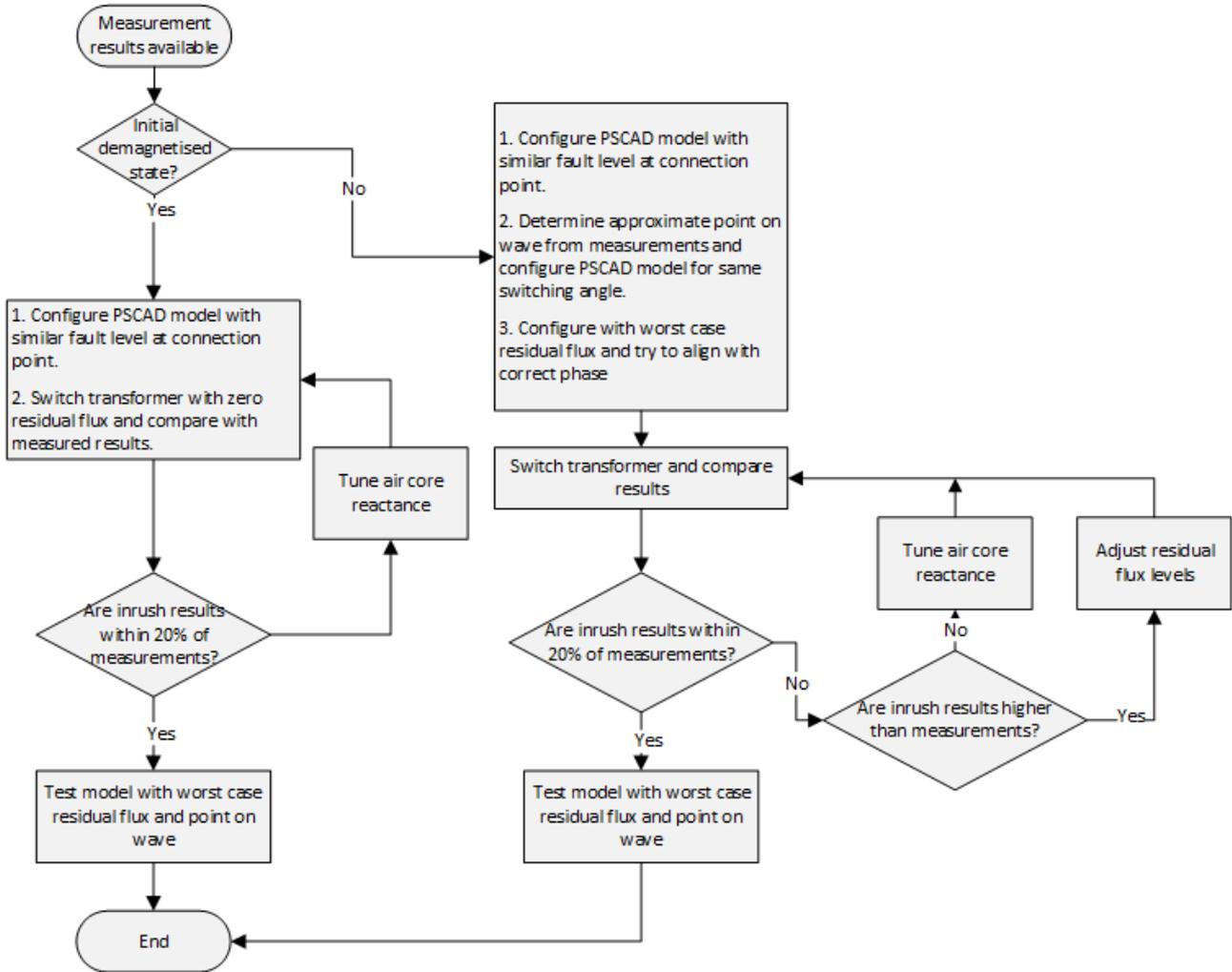
Figure 20 - Model validation flowchart
