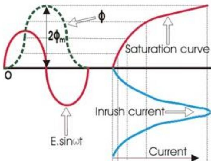
Figure 4 - Inrush Current vs Saturation Curve vs Applied Voltage<sup>3</sup>
