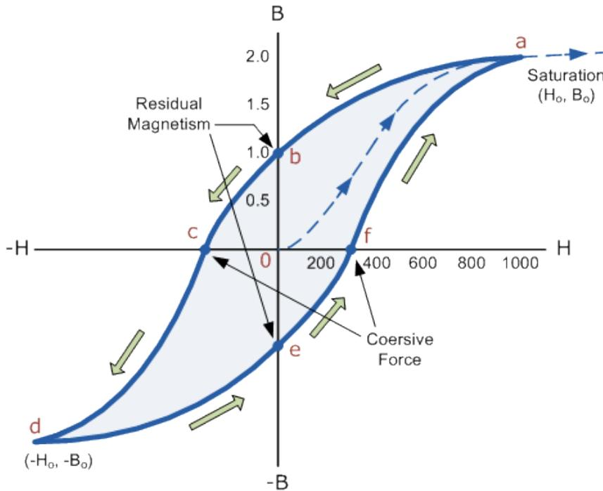
Figure 7- Hysteresis Loop for Magnetism (Electronics Tutorials n.d.)<sup>10</sup>
