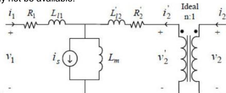
Figure 5 - Classical Approach - Transformer Model<sup>6</sup>
