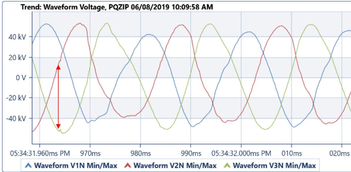
Figure 16 – Measured instantaneous line to neutral voltages
