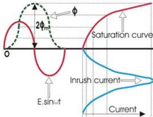
Figure 8- Inrush Current vs Saturation Curve vs Applied Voltage<sup>11</sup>
