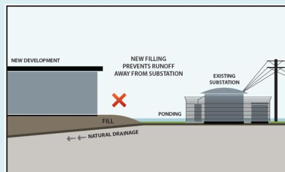
Filling works on adjoining landholdings could cause pooling of water on substation sites which were previously flood free. Fill works can create 'dam walls', obstructing the natural/existing flow of water through a site. This can significantly impact on the safe operation of our electrical infrastructure.
