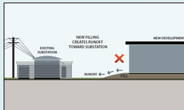
Filling or excavation works could alter existing overland flow and flood paths if managed poorly. The works can impact on the continued safe operation of a substation by reducing its flood immunity.
