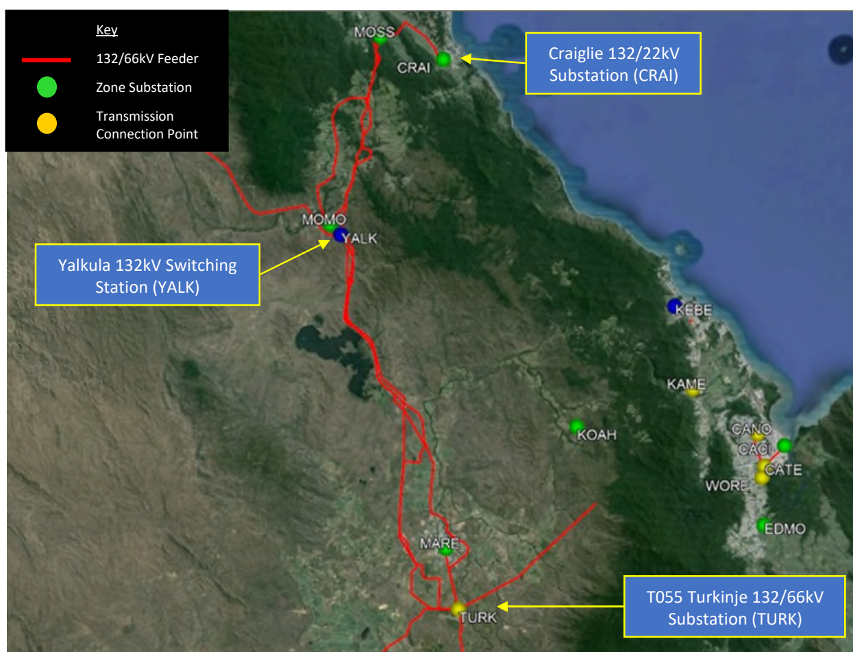
Figure 1: Existing network arrangement (geographic view)
