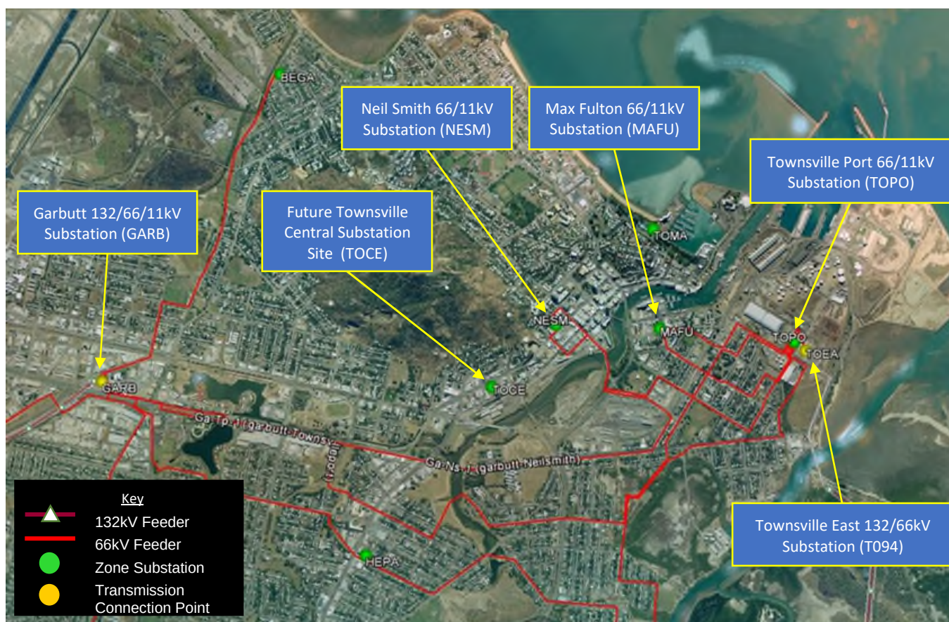
Figure 1: Existing network arrangement (geographic view)
