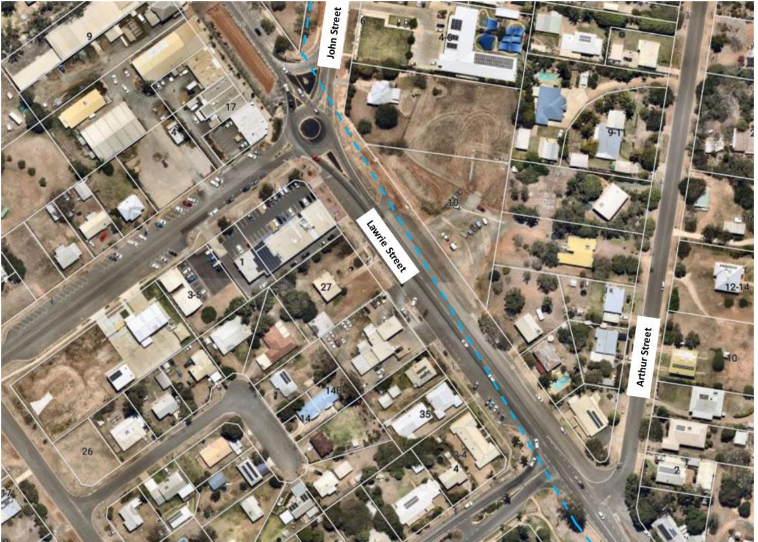
Fig 2 – The line route for the new underground 66kV cable under Lawrie Street between John Street and Whitman Street.
