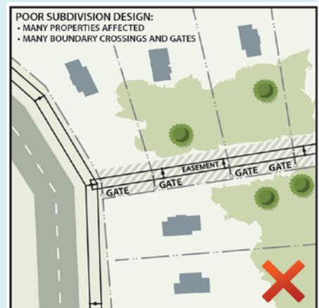
Figure 1: Integrating powerlines into new developments should never compromise the safety and efficiency of the electricity network, particularly access to an easement.
