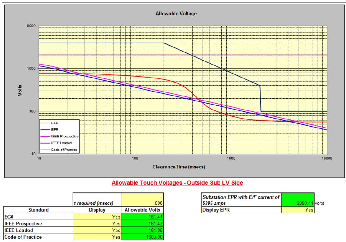
**Figure 8: Max Allowable Prospective Voltage versus Time**
