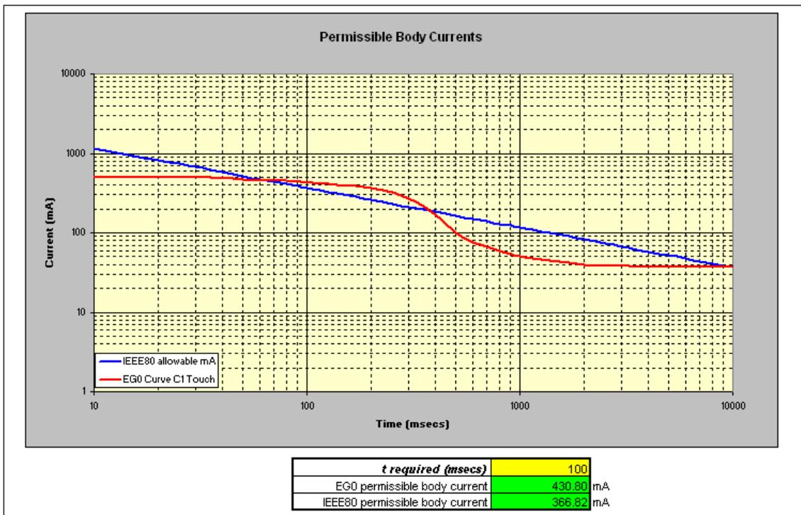
Figure 9: Max Permissible Body Current versus Time
