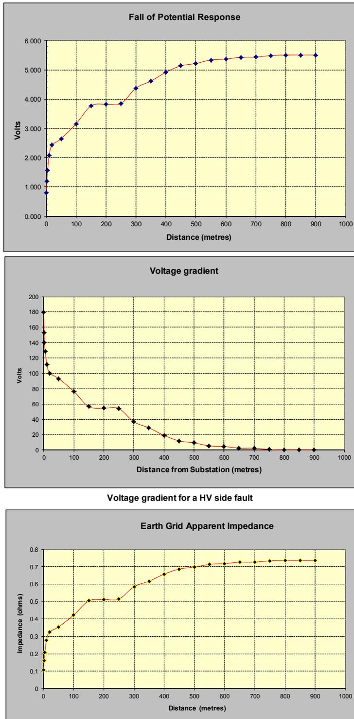
**Figure 4: Voltage Gradient Plots**
