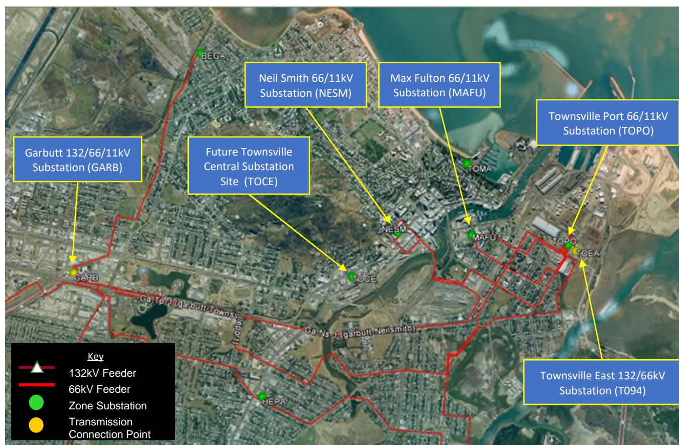
Figure 1: Existing network arrangement (geographic view)
