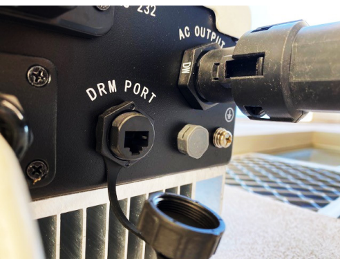
Demand Response Mode (DRM) plug on inverter
