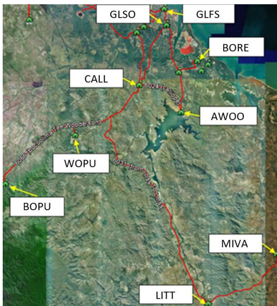
Figure 1: Existing 66kV network arrangement (geographic view)
