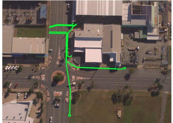
Fig 4 – Cable recovery and reinstatement path along Gordon Street to the east.
