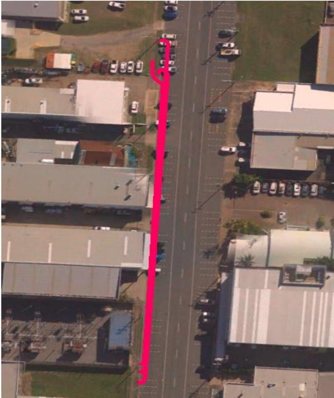
Fig 3 – Excavation path for conduit trenches that will house the high voltage cables out of the substation down to Victoria Street.
