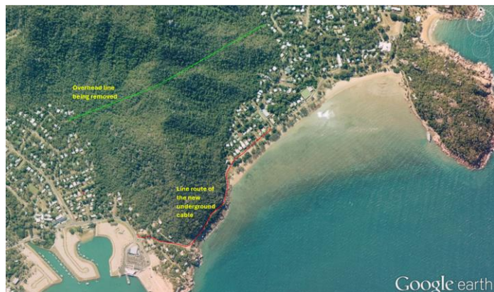
Fig 2 – The line route for the new underground cable and the location of the powerline being removed from the National Park.
