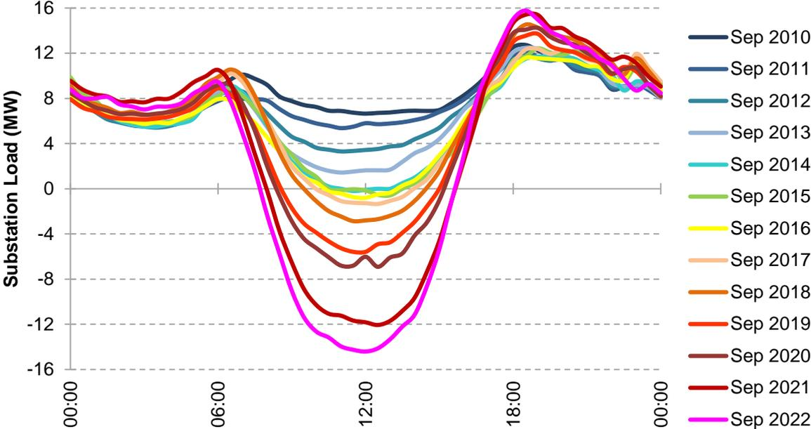
The increase in Embedded Generation (EG) on our feeders makes it more challenging to identify underlying load growth, as additional daytime load can be offset by local generation. Variation to electricity use patterns or growth in load only becomes fully apparent when an unexpected event causes the solar PV systems to stop generating.
