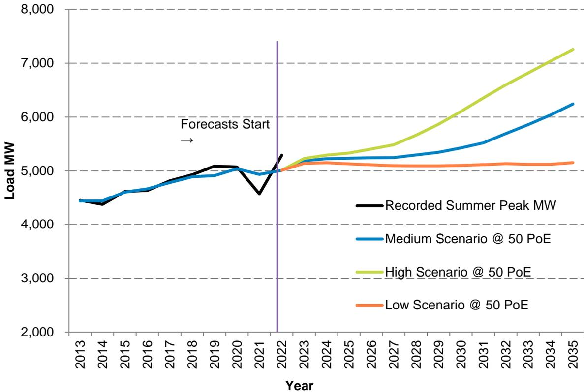
Energex Summer system peak MW demand hit a historical high of 5,289MW over 2:30 ~ 3:00 pm on 2nd-Feb-2022 as the temperatures at Amberley hit a maximum of 33.4 degrees Celsius. This peak is 15.7% higher than the previous year due to the combination seasonal intensity varying significantly between last year and this year, and the government response to COVID-19 boosting the economy.
