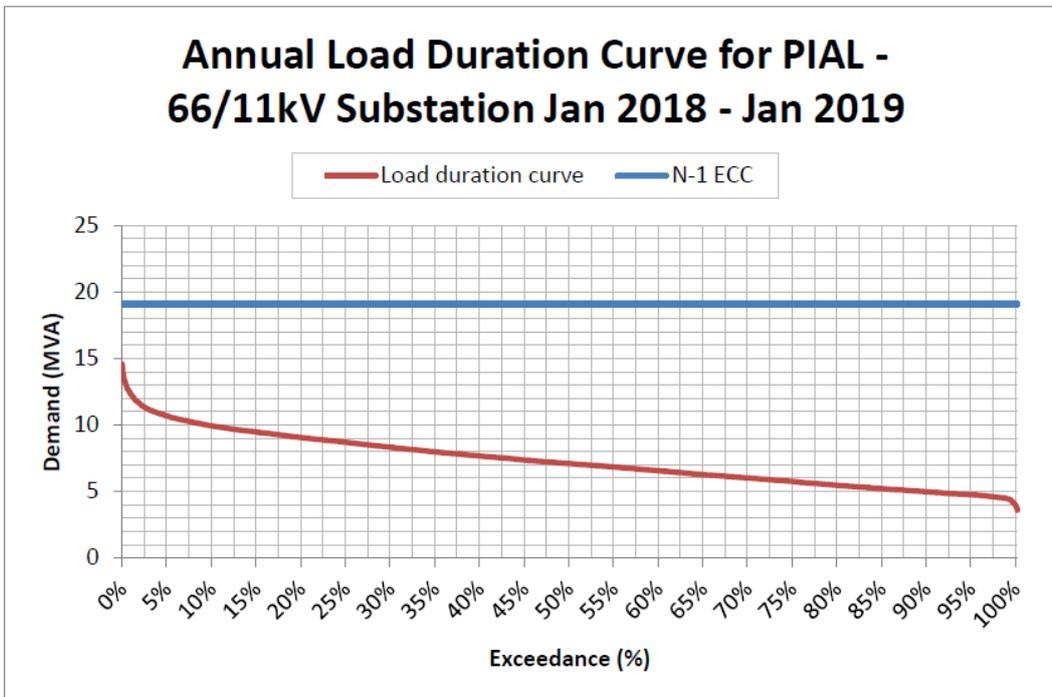
Figure 3 – Pialba substation load duration curve
