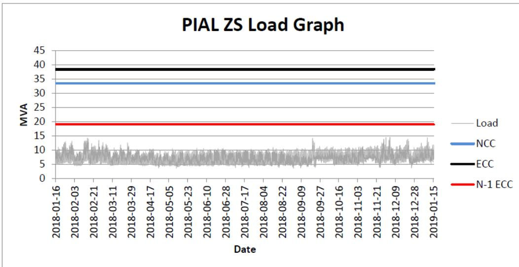
Figure 2 – Pialba substation load
