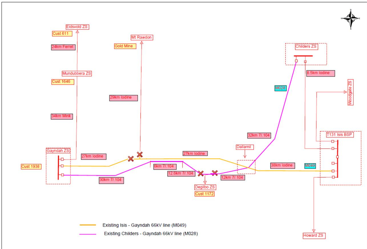
Figure 2 - 66kV Subtransmission Network Representative Geographic Diagram
