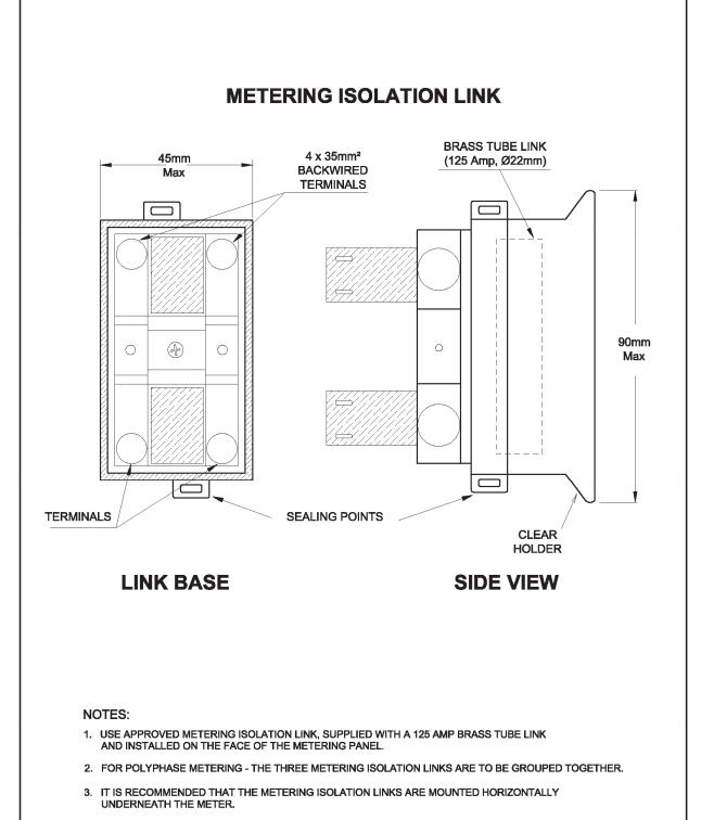
4. CLEARANCE OF 40mm TO BE LEFT AT EACH END OF LINK TO FACILITATE SEALING.
